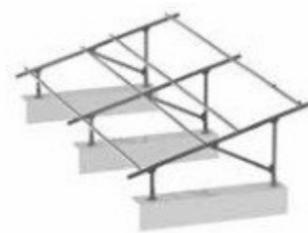
**4.** Put the rail on the rack and fix the panel by end clamp and mid clamp
